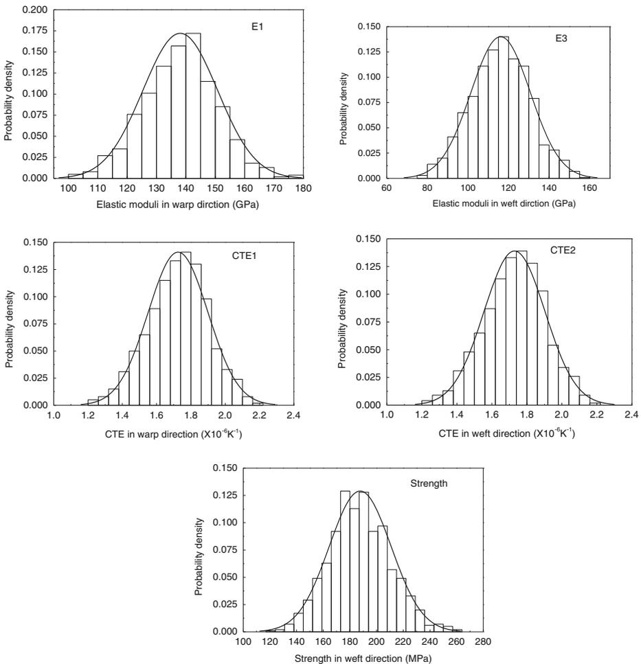
**Fig. 4** Probability density distributions of mechanical and thermal properties of 2.5D C/SiC composite
