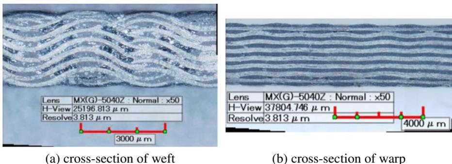
**Fig. 1** Cross-section of 2.5D C/SiC composites **a** cross-section of weft **b** cross-section of warp
