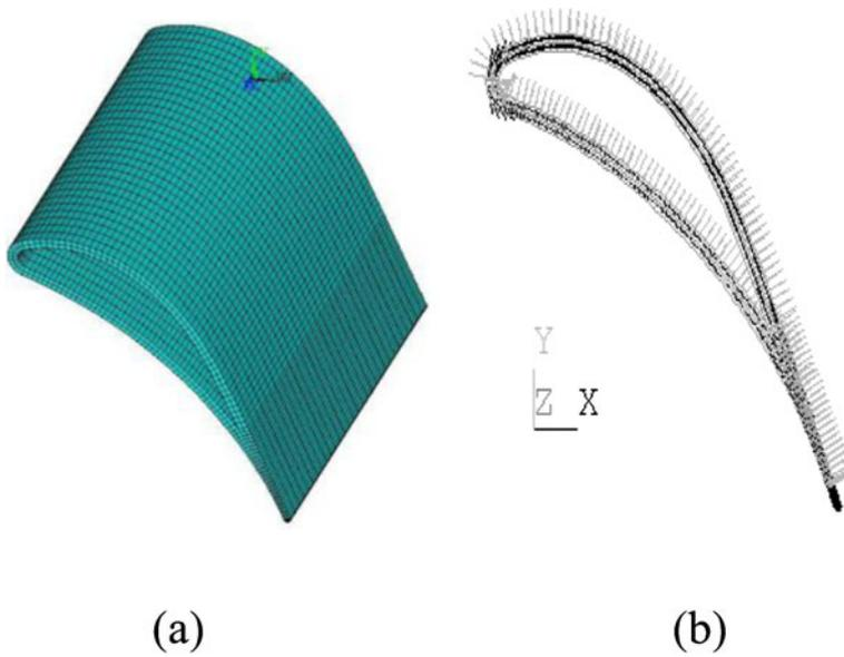
**Fig. 5** Finite element model and mesh generation of turbine stator vane
