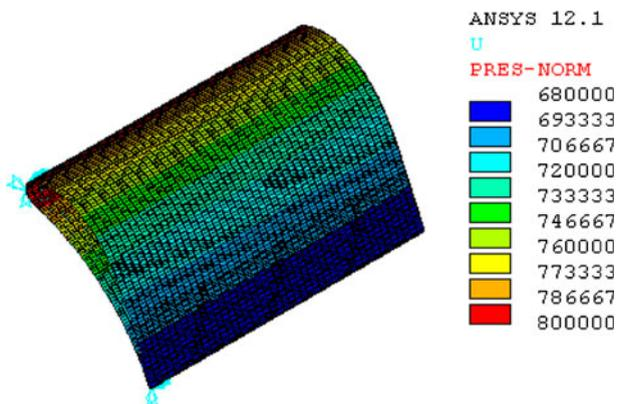
**Fig. 6** Pressure distribution of turbine stator vane
