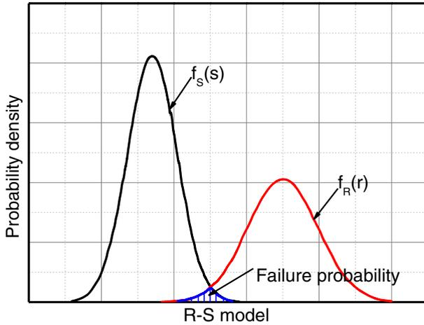
Fig. 10 Failure probability model
