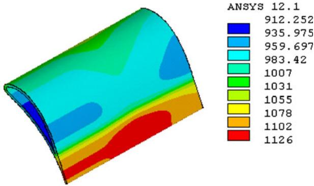
Fig. 7 Temperature distribution of turbine stator vane
