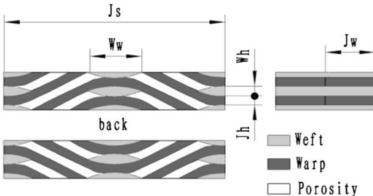
Fig. 2 Microstructure of 2.5D C/SiC composite
