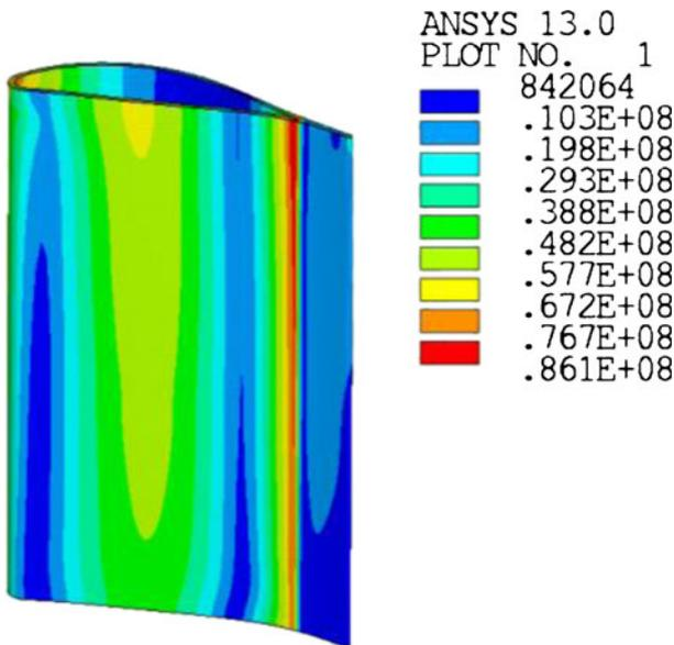
Fig. 8 Stress distribution of turbine stator vane
