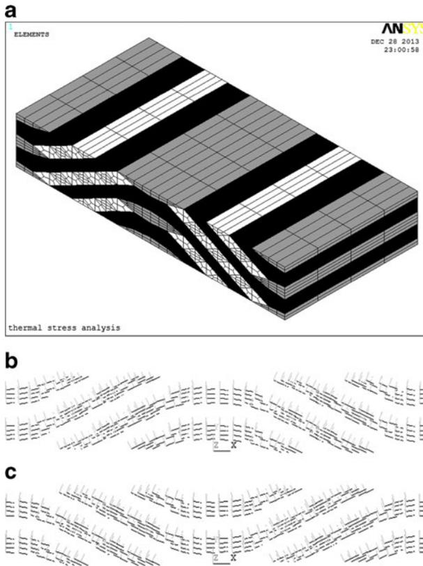
**Fig. 3** Finite element models of 2.5D C/SiC composites **a** Finite element model of 2.5D composites **b** Longitudinal direction of front part **c** Longitudinal direction of back part
