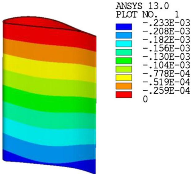
**Fig. 9** Radial deformation of turbine stator vane
