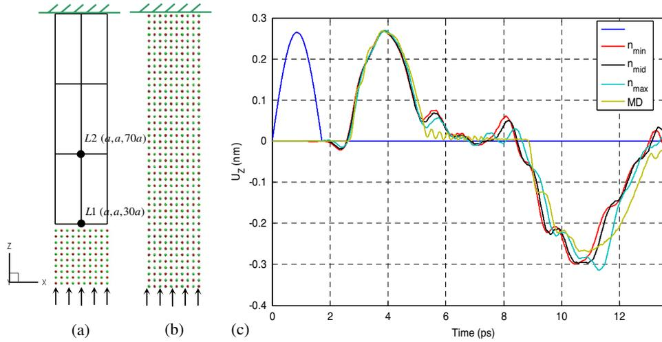
**Figure 4.** Wave propagation through the interface between the atomic region and the continuum region. The computational model of AFT and MD under a compressive impulsive loading is illustrated in (a) and (b), respectively. Displacement response of Point L2 ( $a, a, 70a$ ) under the loading with the frequency  $\omega \approx 1.6$  THz is shown in (c).
