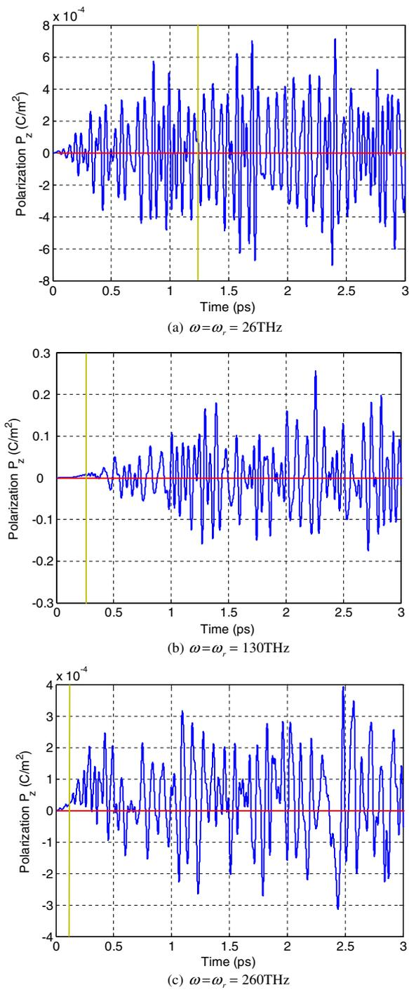
**Figure 9.** Polarization  $P_z$  versus time under different frequencies.
